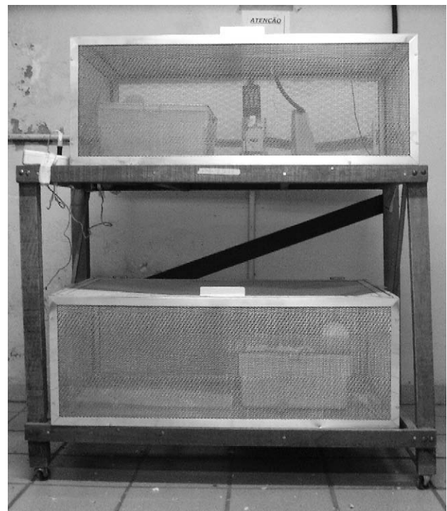
Fig. 1. UHF-EMF exposure set-up. In this picture, the UHF-EMF Faraday cage is over the control Faraday cage. Inside the UHF-EMF Faraday cage, the plexiglass cage and the analogue cellular phone can be seen.
