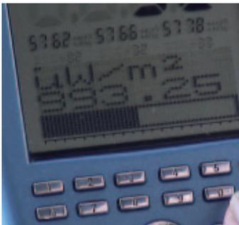
With the setting "pulse" and a span of 5760-5780 MHz, the Spectran HF 6080 Rev.3 finds ghost frequencies up to 993  $\mu\text{W}/\text{m}^2$ , which do not exist in reality.
