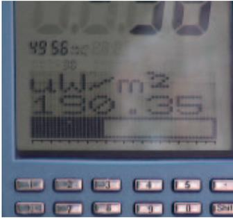
With the setting "no pulse" and a span of 4940-4960 MHz, the Spectran HF 6080 Rev.3 finds a ghost frequency at 4956 with over 190  $\mu\text{W}/\text{m}^2$ .
