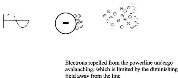
Fig. 1 Schematic outline of the formation of powerline corona ions.
